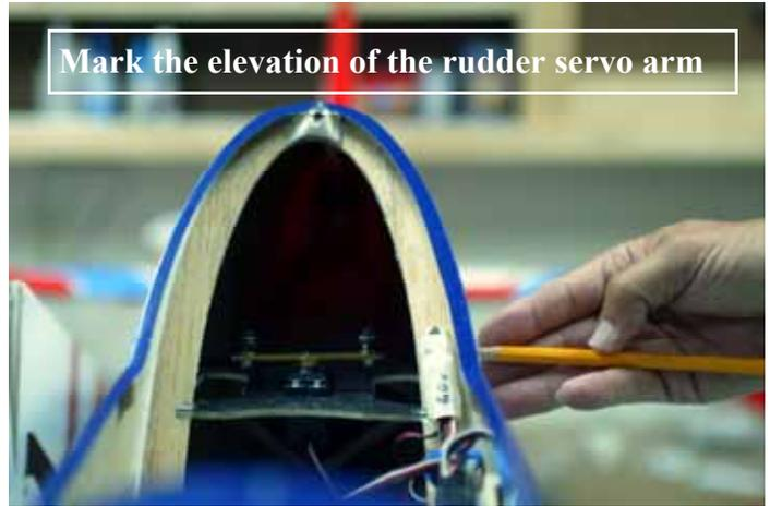
Mark the elevation of the rudder servo arm
