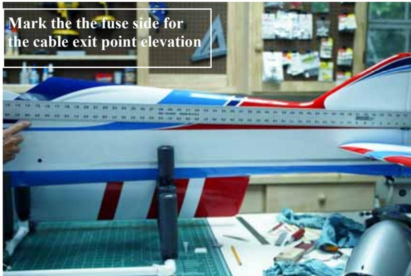
Mark the the fuse side for the cable exit point elevation
