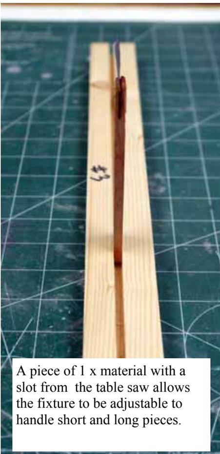
A piece of 1 x material with a slot from the table saw allows the fixture to be adjustable to handle short and long pieces.
