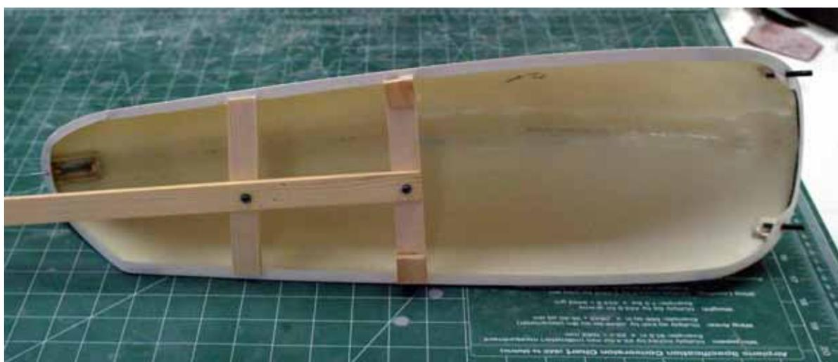
To use, just slide the slots in the end of the cross pieces over the flanges on the chin cowl or canopy. When the part is painted, set the fixture on a flat surface for drying.
